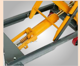
▶ Hydraulic lifting and lowering device
